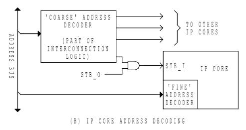
*Illustration* 8-22: *WISHBONE* partial address decoding technique
