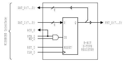
*Illustration 8-9: Simple 8-bit WISHBONE SLAVE output port*
