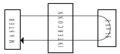
*Illustration 4-1: Asynchronous cycle termination path*
