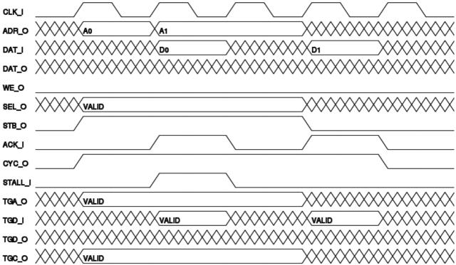
Illustration 3-11: Pipelined BLOCK READ cycle
