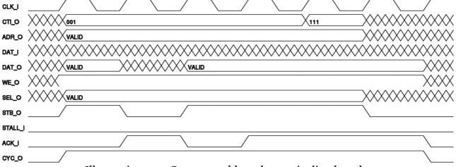
Illustration 4-9: Constant address burst pipelined mode
