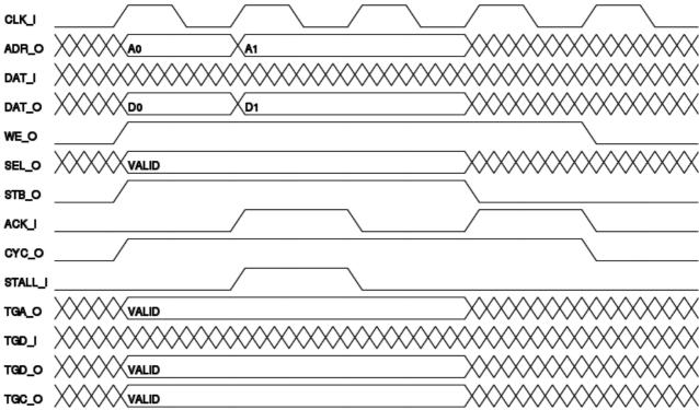
Illustration 3-13: Pipelined BLOCK WRITE cycle
