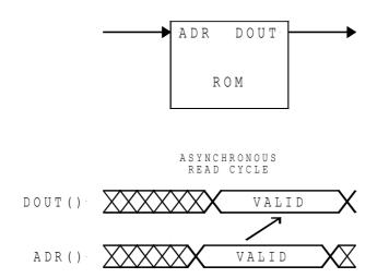
Illustration 8-13: FASM asynchronous ROM connection and timing diagram
