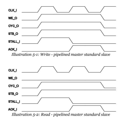
This logic could be implemented in a wrapper. The new top level module would present a pipelined peripheral. In Verilog HDL this could optionally be done in the port mapping.
