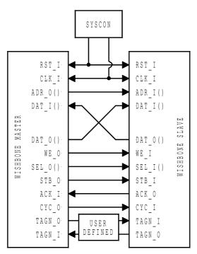
*Illustration 1-2: Standard connection for timing diagrams.*
