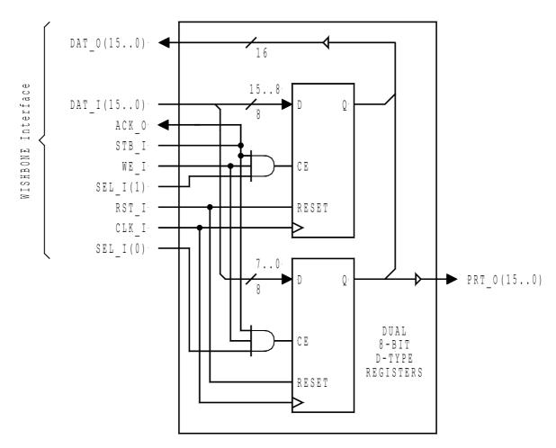
Illustration 8-11: Simple 16-bit WISHBONE SLAVE output port with 8-bit granularity
