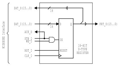
Illustration 8-10: Simple 16-bit WISHBONE SLAVE output port with 16-bit granularity
