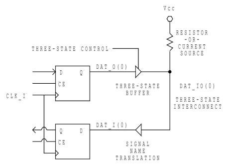
*Illustration* 8-18: *Connection of a data bus bit to a three-state interconnection*
