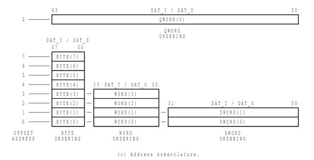
*Illustration 3-15: Operand locations for input and output data ports*
