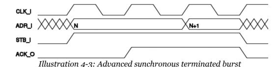
During cycle-1 the MASTER initiates a transfer. The addressed SLAVE responds in the next cycle with the assertion of ACK\_O. The MASTER starts a new transfer in cycle-3. The SLAVE knows in advance it is being addressed again, therefore it keeps ACK O asserted.
