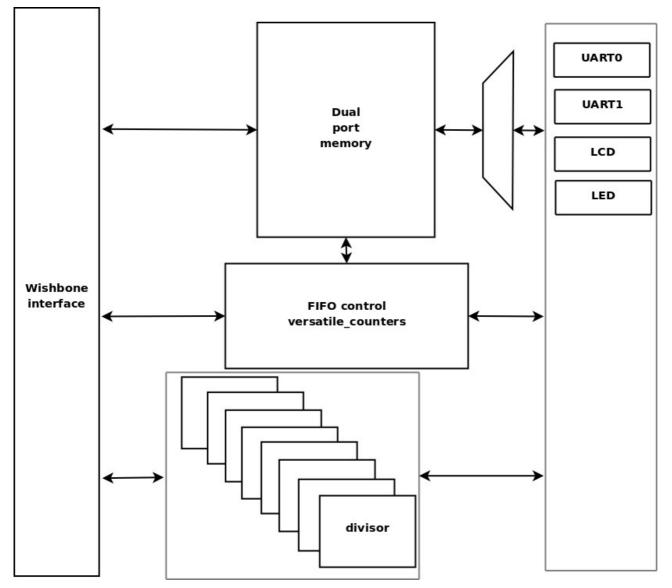
The basic idea behind this IP is that multiple, 8 by default, IO functions share a dual port memory used as multiple FIFO channels. On the system side all IO functions share a common wishbone interface.
